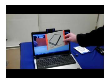
Each color coded card corresponds to a particular item. When the card is shown to the camera, the vision algorithm determines which color it is being shown based on an RGB threshold. Once the color has been determined, the vision algorithm determines which object this color corresponds to, associates the object with the color, and then sends a message to the RobBot to retrieve that particular object.
